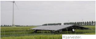
Self driving solar panels for agri solar. For de-central energy (Hydrogen) production at agricultural farms.
