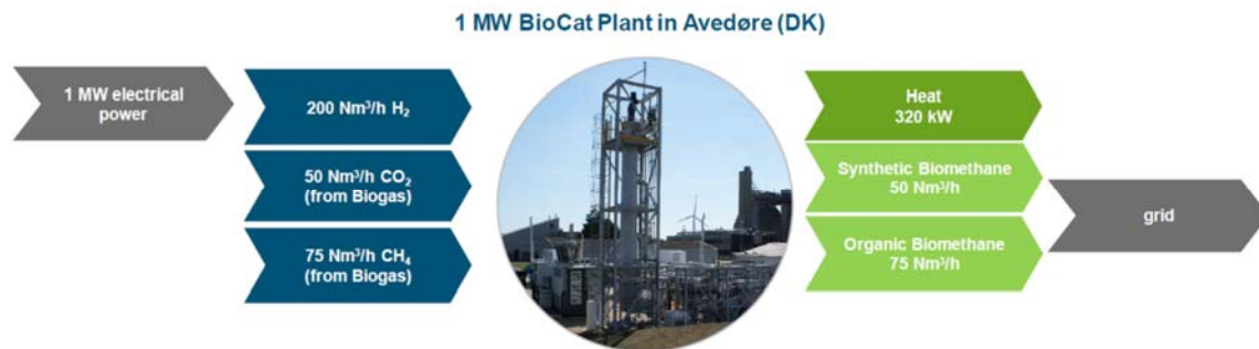
Figure 57. Energy flow in the Electrochea process 142 installed at Avedøre, Denmark. The heat is released at approx. 60°C.
