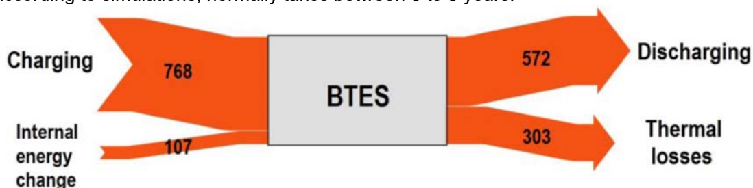
Figure 67 181 . Heat balance for the BTES in Brædstrup for the period 2014-2017, numbers in MWh.
