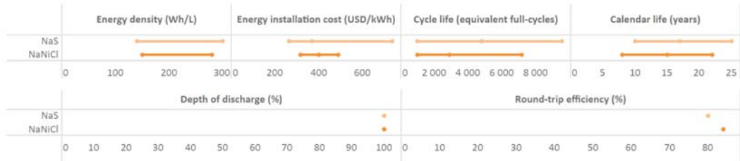
Figure 45: Properties of high-temperature battery electricity storage systems, 2016
