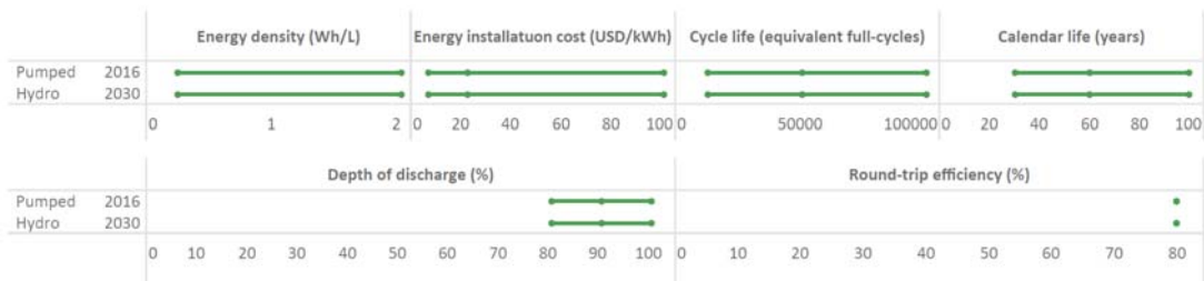
Figure 16: Properties of pumped hydro storage systems, 2016 and 2030
