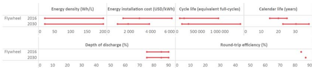
Figure 22: Properties of flywheel energy storage systems, 2016 and 2030
