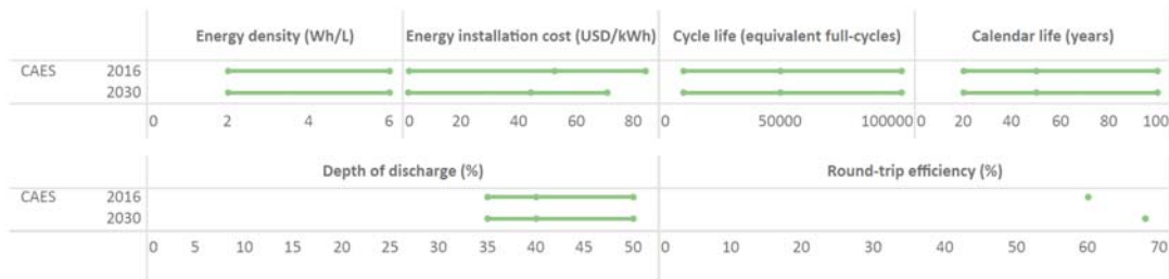
Figure 19: Properties of compressed air energy storage systems in 2016 and 2030
