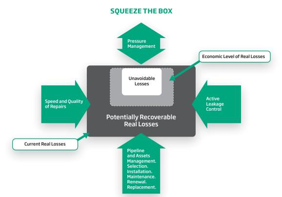
Standard illustration of potential reduction of real losses through four types of activities; pressure management, speed and quality of repairs, active leakage control and pipeline and assets management.
